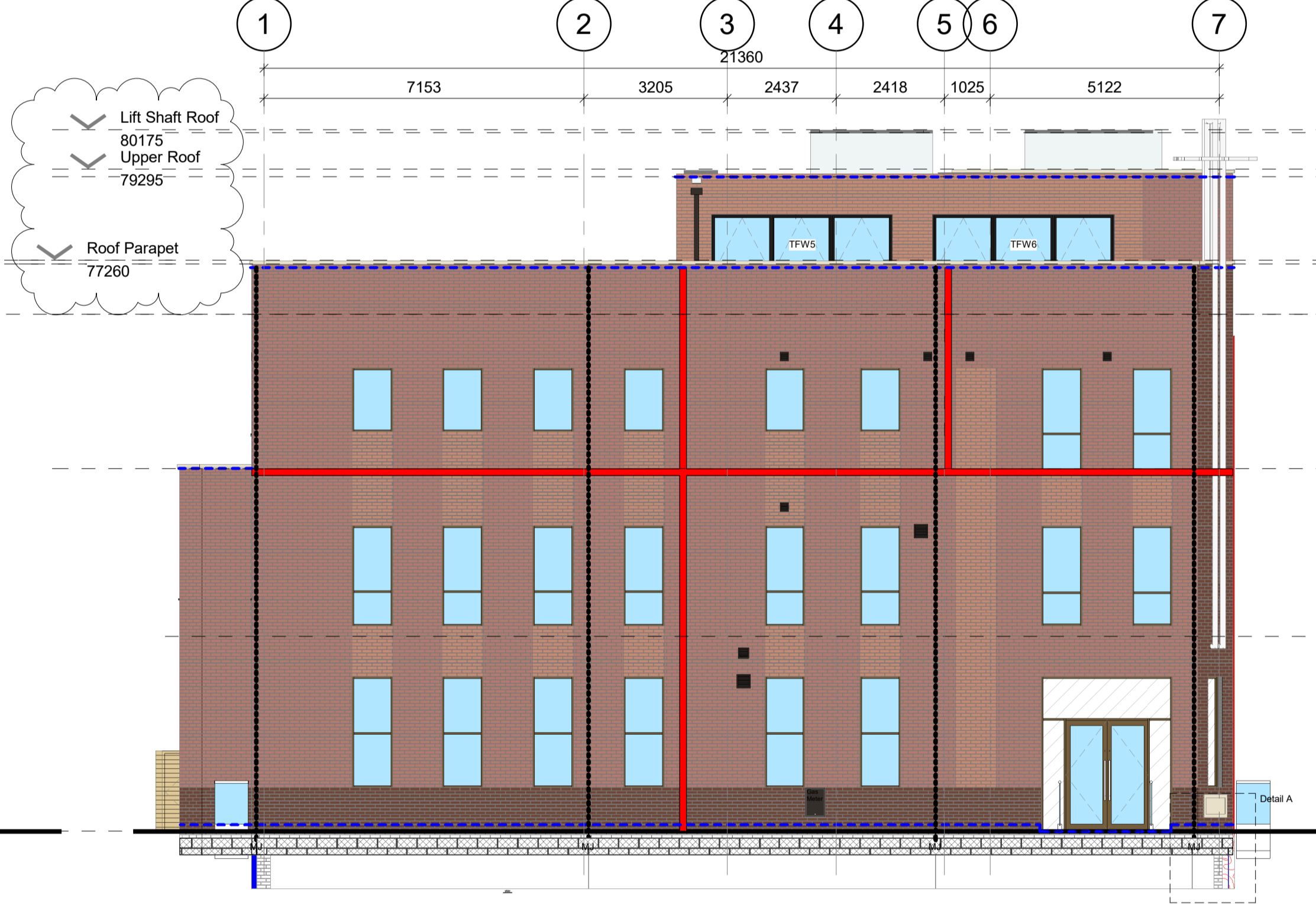
Elevation D (South) Construction 1 : 100
